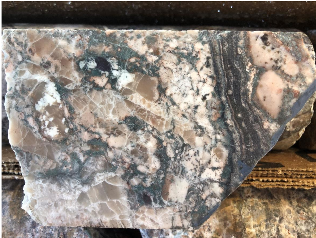
Figure 3. Photograph of altered iron oxide breccia in Hole 5 in the center of the ZTEM conductive pipe at Hemco. Hydrothermal breccia at 153 metres is cemented by specularite and silica. Breccia clasts are intensely sodic and potassically altered diorite. For scale, HQ drill core = 6.4 centimetres across.
