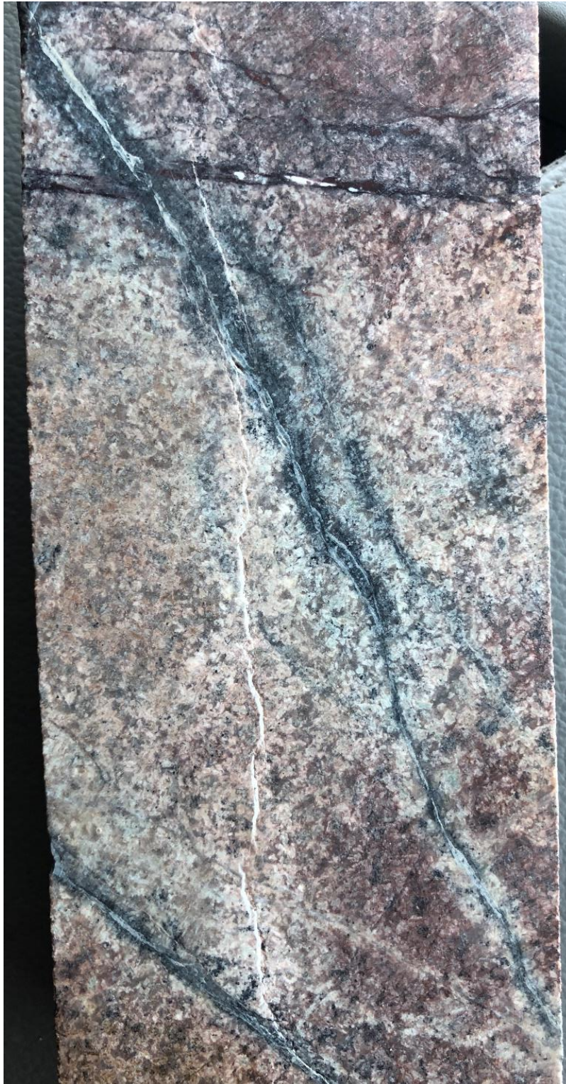
Figure 5. Stockwork of quartz-hematite-sericite veins in phyllic alteration in Hole 7 (57 metres). Phyllic veins are characterized by disseminations of pyrite and chalcopyrite within the veins, and sericite selvage on the vein margins. The complete replacement of host rock sodic diorite by sericite-albite-hematite in this photo is characteristic of the first 100 meters of Holes 6, 7 and 8. For Scale, HQ drill core = 6.4 centimetres across.
