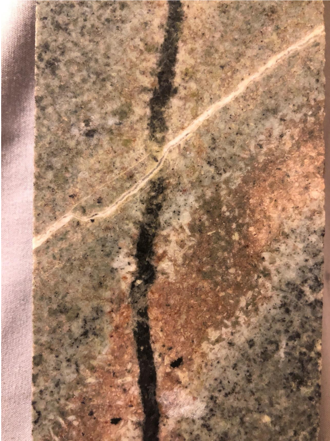
Figure 6. Hydrothermal biotite veins characteristic of pervasive calc-potassic alteration in Hole 8 (240 metres). Host sodic diorite is completely replaced to an alteration assemblage of albite-K feldspar-biotite-magnetite. Disseminated chalcopyrite and bornite copper sulfides are in the pink potassium feldspar replacement band cut by the 5 mm wide hydrothermal biotite vein. For scale, HQ drill core = 6.4 centimetres across.
